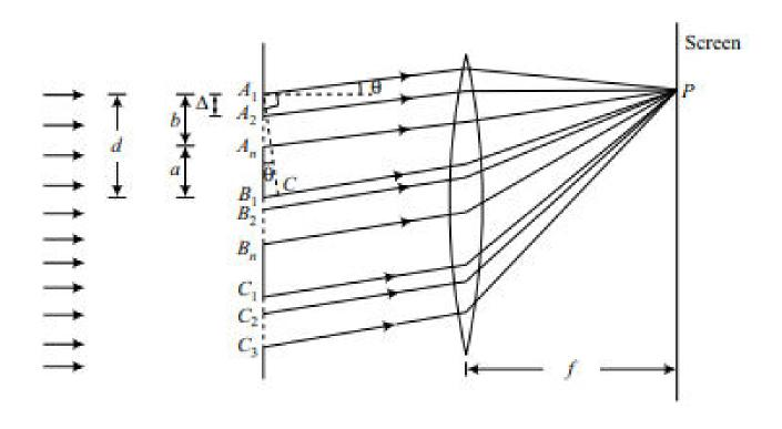
$$E = A \frac{\sin\beta}{\beta} \cos(\omega t - \beta) + A \frac{\sin\beta}{\beta} \cos(\omega t - \beta - \varphi_1) + \cdots + A \frac{\sin\beta}{\beta} \cos(\omega t - \beta - (N - 1)\varphi_1)$$
